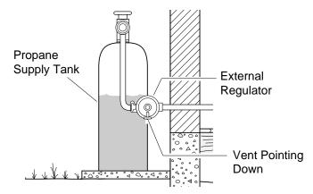
Figure 10 - External Regulator With Vent Pointing Down
